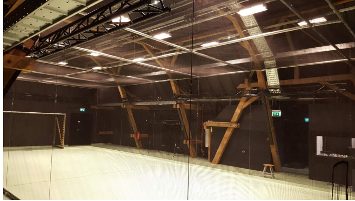
Fig. 1: Imaging Facility for Data Acquisition. The system consists of six Vue 2, four Vantage 5 and 26 Vero 2.2 sensors covering a volume of approximately 15 \times 7 \times 4 meters. © CASCB Uni Konstanz.
